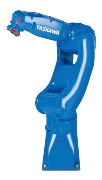
The MOTOMAN GP8 is an extremely fast and precise 6-axis industrial robot with a payload capacity of up to 8 kg. With a reach of 727 mm and a high repeatability of  $\pm$  0.02 mm, it is ideally suited to assembly tasks, but also universal handling tasks, CNC machine tool tending or packaging. Its smooth, streamlined and award-winning modern industrial design is attractive and minimizes the space requirements at the installation site.
