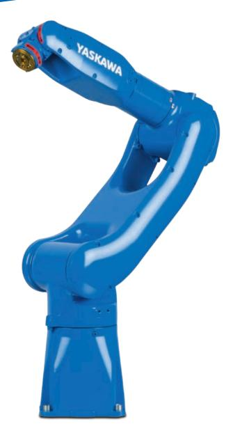
The MOTOMAN GP7 is an extremely fast and precise 6-axis industrial robot with a payload capacity of up to 7 kg. With a reach of 927 mm and a high repeatability of  $\pm$  0.03 mm, it is ideally suited to assembly tasks, but also universal handling tasks, CNC machine tool tending or packaging. Its smooth and streamlined modern industrial design is attractive and minimizes the space requirements at the installation site.
