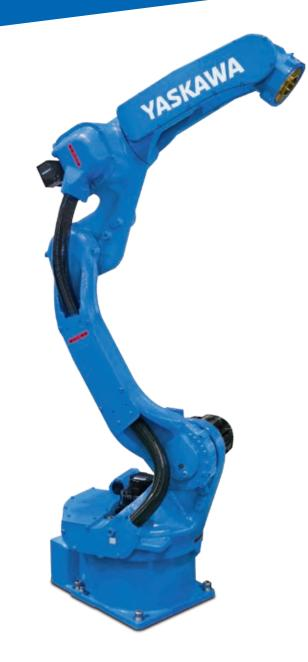
The MOTOMAN GP12 is a fast and precise 6-axis industrial robot with a payload capacity of up to 12 kg. With a reach of 1440 mm and a high repeatability of  $\pm$  0.08 mm, it is ideally suited to assembly tasks, but also universal handling tasks, CNC machine tool tending or packaging. Its streamlined modern industrial design minimizes the space requirements at the installation site.
