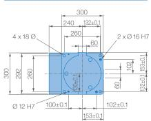
Mounting options: Floor, ceiling, wall, tilt\* Protection class Version YR-1-25VXH12-A00 Standard: Main axes (S, L, U) IP54, wrist IP67 Protection Class Version YR-1-25VXH12-C00: Main axes (S, L, U) IP65, wrist IP67 \* tilt with condition of angle – see table below
