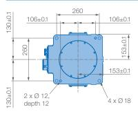
Mounting options: Floor, ceiling, wall, tilt\* Protection class: IP67
